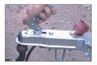
The handle is in the upper position and kept here whilst the hitch is lowered by using the jockey wheel on to the vehicle's tow bar.
