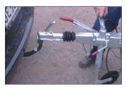
The handle is, in the upper position i.e. open, then the hitch is lowered by using the jockey wheel on to the vehicles tow bar.
